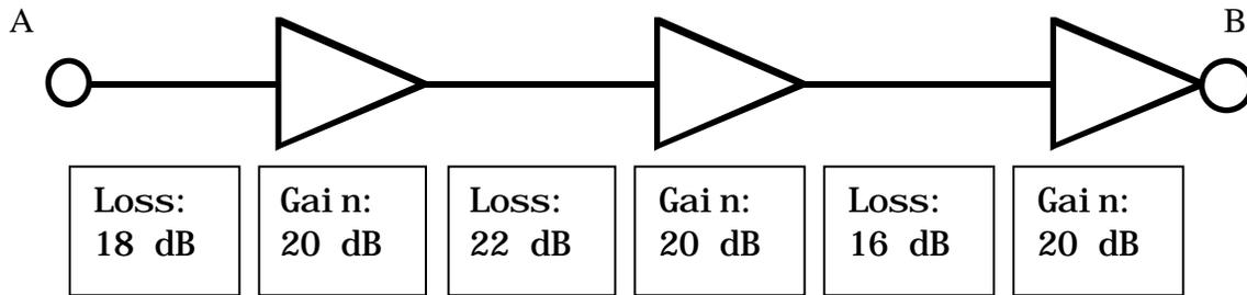
\_\_\_ **4 dB** \_\_\_ What is the overall gain in dB for this transmission system (from A to B)?
